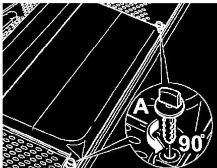
2. Open turn-lock fasteners -A-.
