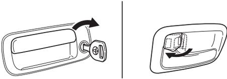
If any door is manually unlocked via Smart Key.
