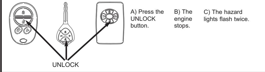
Using Method 1, your vehicle will remain unlocked for 30 seconds. Then it automatically relocks if no doors are opened. If your vehicle will not be in plain view for that time, or you have other security concerns, you may wish to use Method 2 (below), which does not unlock the vehicle.
