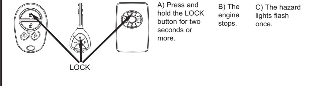
NOTE: All doors will remain locked after the engine is shut off.
