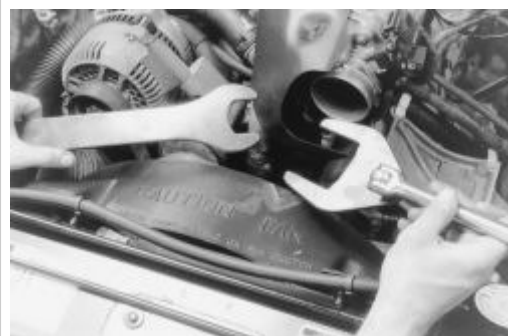
Fig. 5: Remove the air intake tube. You will need these specialized tools to unfasten the fan clutch nut
