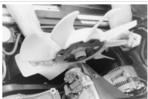
Fig. 7: Remove the fan and clutch assembly from the vehicle
