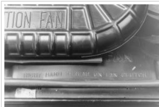
Fig. 4: Before attempting to unfasten the engine fan, check the fan shroud for indications of normal or reverse threads
