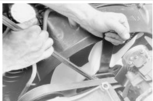
Fig. 6: Using the special tools, loosen the fan clutch nut in the direction indicated on the shroud.
