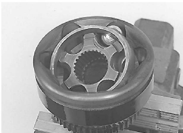
**Note:** Replace the drive shaft assembly if any component has cracking or wear damage. Scratches and minor pitting of the ball tracks are permitted.
