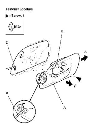
2. Remove the screw from the armrest portion of the door panel. Release the clips that hold the door panel (A) with a commercially available trim pad remover (B), then remove the door panel by pulling it upward, and disconnecting the power window switch connector (C). Remove the door panel with as little bending as possible to avoid creasing or breaking it.
