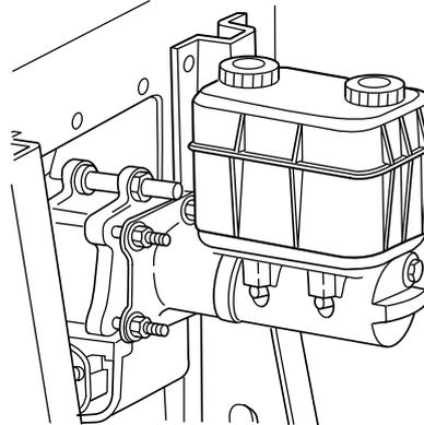
1. Clean the reservoir cap before removal to prevent dirt or water from entering the reservoir.
