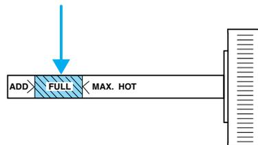
5. If the fluid is low, add fluid in small amounts, continuously checking the level until it reaches the FULL range. Be sure to put the dipstick back in the reservoir.
