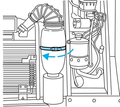
2. Carefully separate the two halves of the air filter housing.
