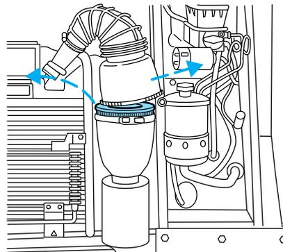
4. Install a new air filter element, ensuring the arrow on the top half of the air filter housing lines up with the notch on the bottom half of air filter housing. Be careful not to crimp the filter element edges between the air filter housing. This could cause filter damage and allow unmetered air to enter the engine if not properly seated.
